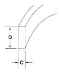
Wearband strip is supplied in 2 materials: 60% bronze filled teflon and phenolic. Phenolic strip is supplied by the foot in coils and the teflon strip is supplied by the inch in roll form.
