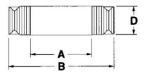
Bearings are made from glass filled nylon with excellent compressive strength. They are used for piston applications between sets of vee packing.
