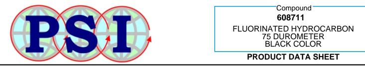
Compound 608711 is a 75 durometer black colored Viton® GF elastomer that is peroxide cured. It exhibits excellent resistance to a wide variety of chemicals including concentrated acid.
