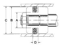
These compact seal assemblies are molded from a specifically blended hybrid material and include a 70 durometer nitrile o-ring expander. They are intergchangeable in many popular TFE piston seal grooves and offer easier installation and better resistance to cold flow and extrusion.
